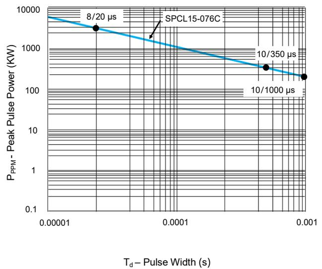
FIGURE 4 Peak Pulse Power Rating Curve
