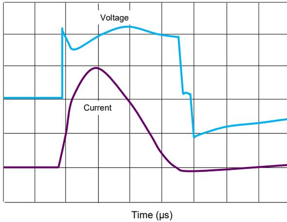
**Note:** The power dissipation causes a change in avalanche voltage during the surge and the avalanche voltage eventually returns to the original value when the transient has passed.
